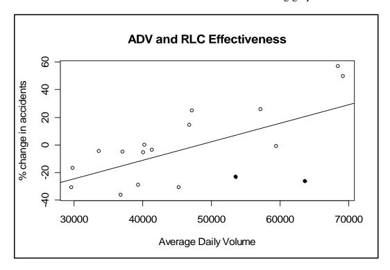
One can see a fairly clear pattern here, with a trend line displayed for reference. The more traffic volume on the road, the more likely RLC placement will be associated with an increase in accidents. Two clear outliers to the trend, labeled with black dots, appear to have high volumes but saw a decrease in accidents after RLC placement. What could account for this? It turns out that these two intersections are "T" intersections.<sup>3</sup>
